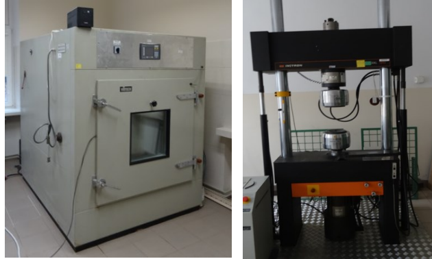
Fig. 2. Vötsch climatic chamber and INSTRON strength machine used in the research (WITPiS materials)
