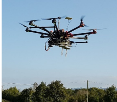
Fig. 4. An example of the GPR system installed on a multirotor UAV platform [40]
