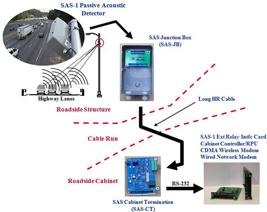
Fig. 7. Diagram of the SAS-1 device concept [13]
