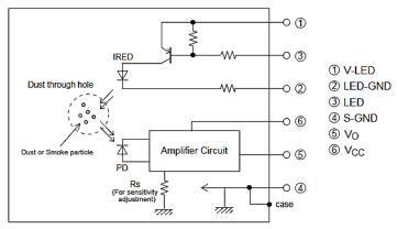
Fig. 26. Sharp GP2Y1010AU0F Diagram [13]
