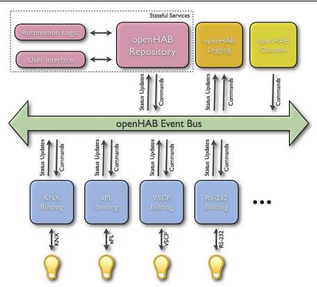
Fig. 10. General scheme of openHAB server operation [6]
