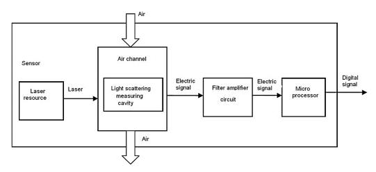
Fig. 12. Functional block diagram of PMS5003 sensor [7]
