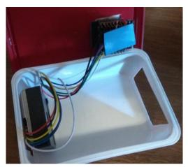
Fig. 29. Inside of dust sensor module of the Smart Wagon system (author's picture)
