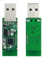
Fig. 8. Texas Instruments ZigBee Network Controller (CC2531) [5]
