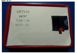
Fig. 28. Dust sensor module of the Smart Wagon system (author's picture)
