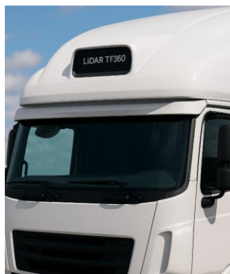
Fig. 4. Visualization of Sensor Placement within the Roof Fairing. Author's Own Elaboration
