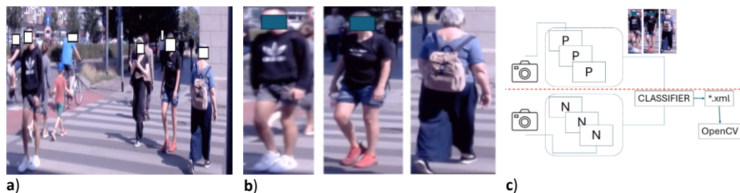
Fig. 1. Haar classifier illustration: a) source material, b) positive image, c) principle of classification. Source: elaboration own
