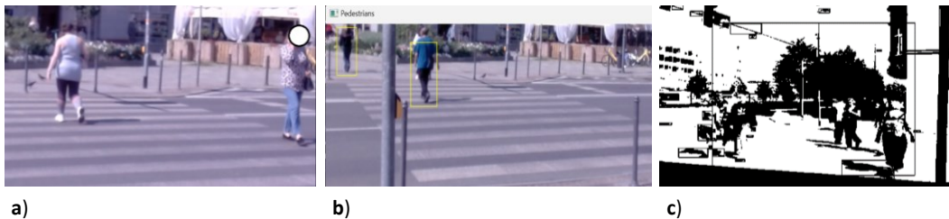
a) b) c) Fig. 5. Cropping and transformatting scene: a) cropping, b) blurred, c) OTSU transformation. Source: elaboration own
