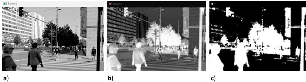
Fig. 6. Digital transformation of scene: a) gray scale, b) negative image, c) thresholding (172,255). Source: own elaboration
