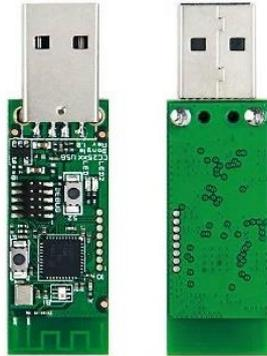
Fig. 8. Texas Instruments ZigBee Network Controller (CC2531) [5]
