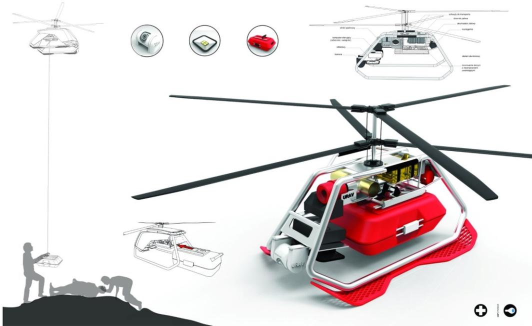
Fig. 10. Unmanned Aerial Rescue Vehicle (UARV) [20]
