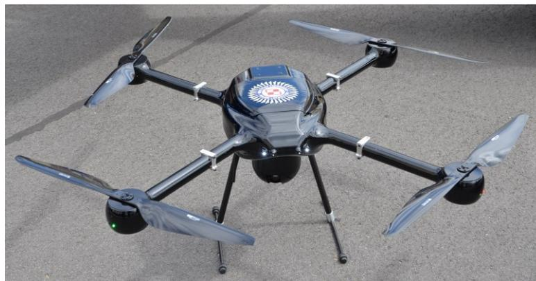
Fig. 9. Vertical Take Off and Landing Unmanned Aerial Vehicle ATRAX [19]
