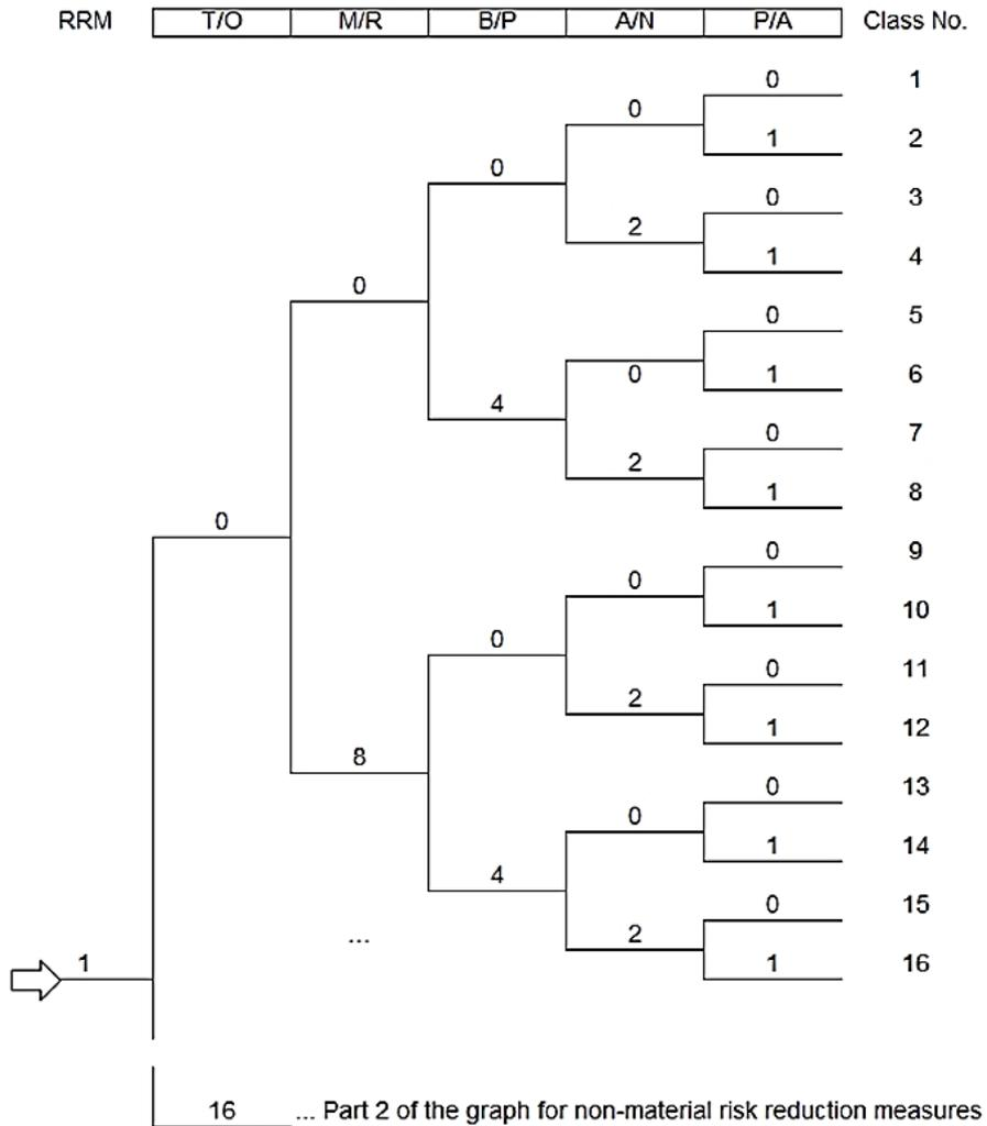
**Fig. 2. Part of the risk reduction measure classification diagram concerning technical measures with rank numbers of their qualities, where: RRM – risk reduction measure; T/O, M/R, B/P, A/N, P/A – symbols of risk reduction measure characteristics: technical/organisational, mechanical/manual, direct/indirect, automatic/non-automatic, passive/active, respectively**
