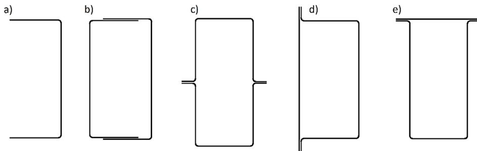
Fig. 3. Types of profiles most often used for the construction of longitudinal beams of independent support frames in delivery vehicles and lorries. A – c-beam, B – double c-beam, C - double hat profile, D – hat profile closed with flat plate on the side, E – hat profile closed with flat plate on top
