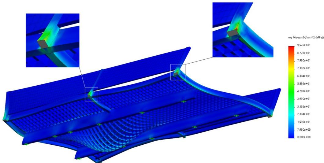
Fig. 17. Map of reduced stresses in the structure of the composite open body under load in the form of a pallet with a weight of 14 kN, dry weight of the structure for the installation of tarpaulin, centrifugal force of inertia and the pressure force of side wind with a direction consistent with the force of inertia of 4800 N
