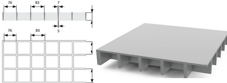
**Fig. 15. Composite support grating plate of the body**
