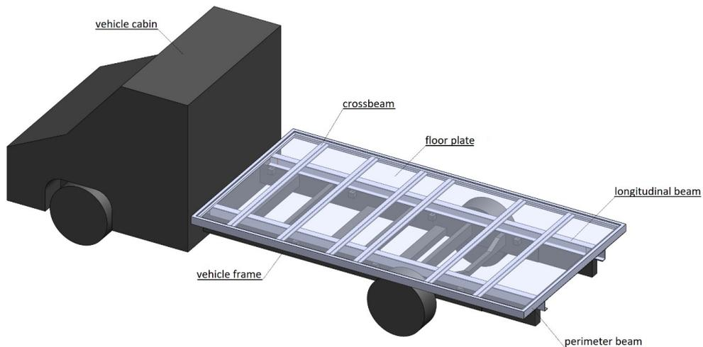
Fig. 6. Diagram of the structure of a classic frame body's floor plate
