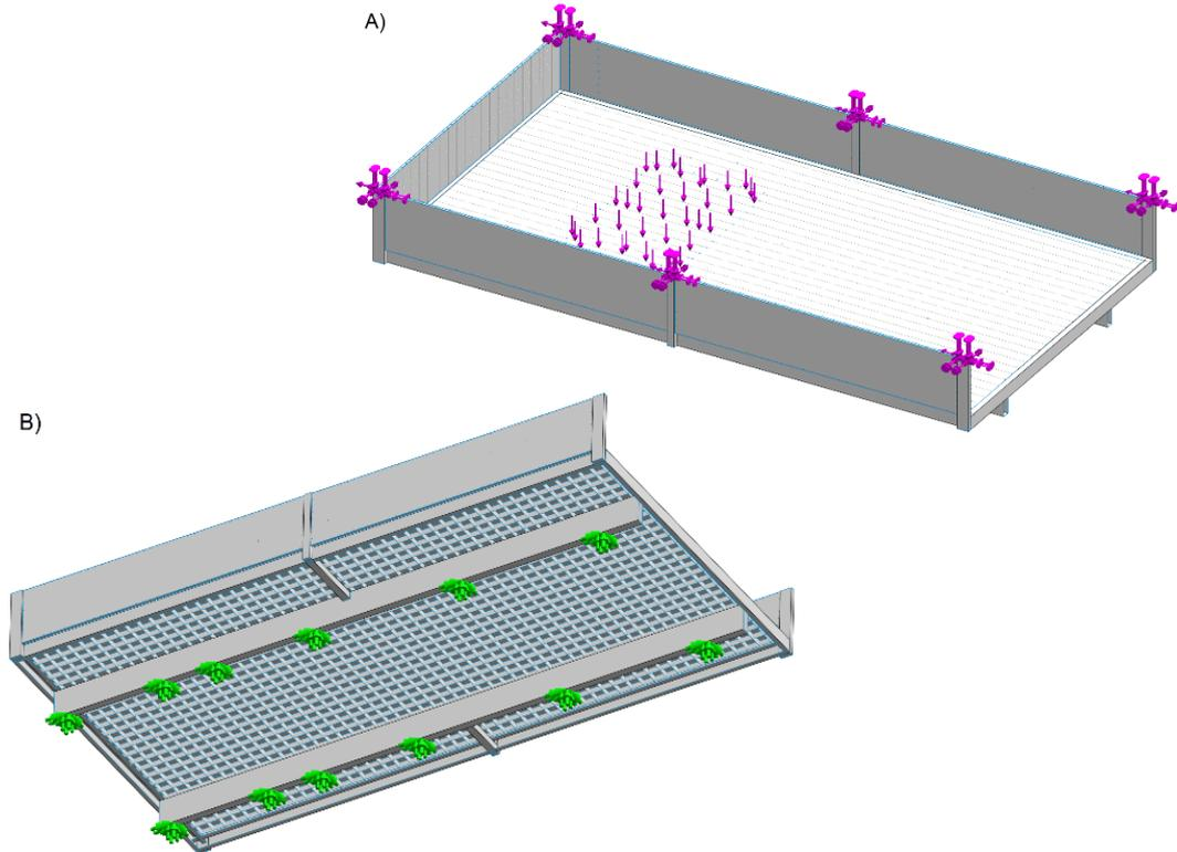
**Fig. 16. The diagram of the boundary conditions applied to body frame. A – view from top, B - view from bottom**
