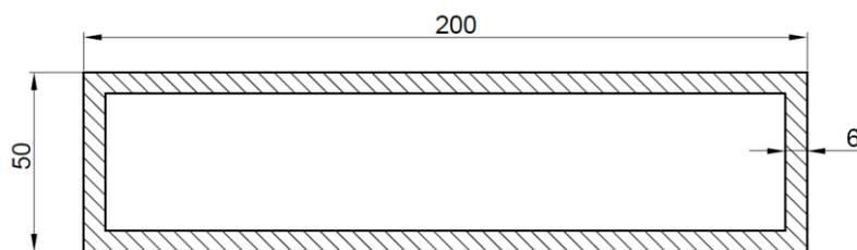
Fig. 14. Cross-section of the longitudinal beam
