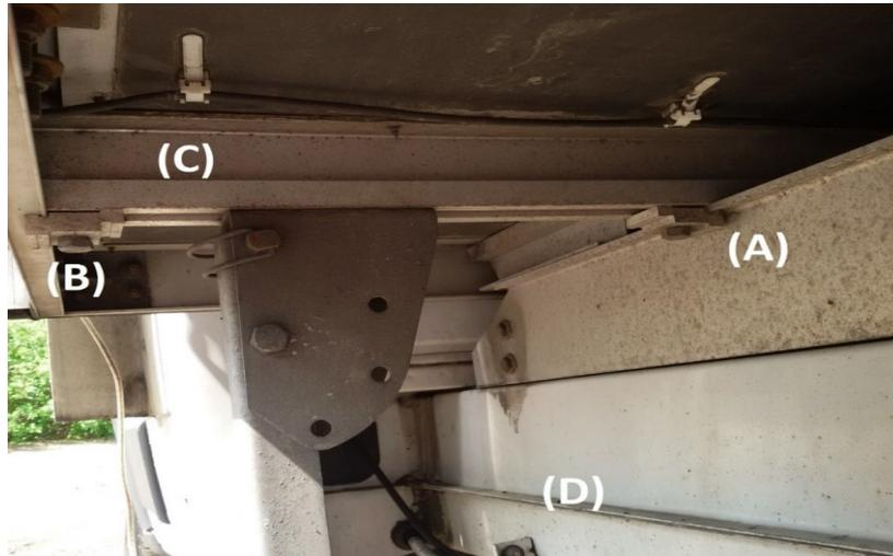
Fig. 7. Example of a body design solution in a Fiat Ducato. A - longitudinal beam of the body frame, B - perimeter beams, C - crossbeam, D – side member of the vehicle support frame. Visible threaded connections of elements
