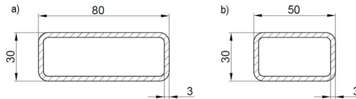
Fig. 12. Cross-sections of support pillars of the open body. a/ corner, b/ middle
