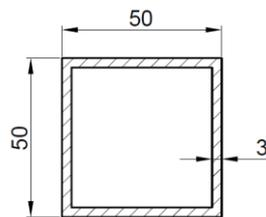
Fig. 13. Cross-section of a beam that strengthens the fastening of the central pillar
