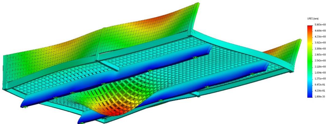
Fig. 18. Map of displacements of the composite structure of the open body under load in the form of a pallet with a weight of 14.5 kN, dry weight of the structure for the installation of tarpaulin, centrifugal force of inertia and the pressure force of side wind with a direction consistent with the force of inertia of 4800 N
