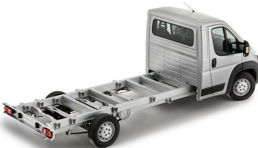
Fig. 4. Standard solution of a support frame on the example of a Fiat Ducato delivery vehicle [13]
