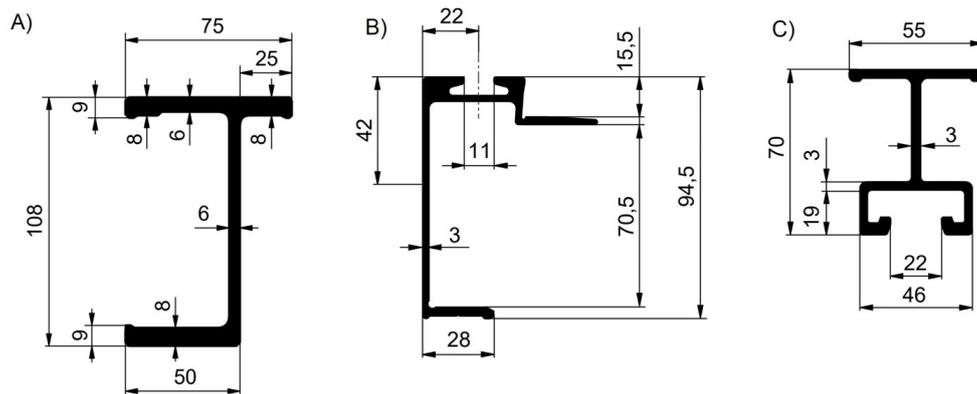
Fig. 8. Examples of cross sections of structural aluminum profiles A - longitudinal beam, B - perimeter beam, C - crossbeam
