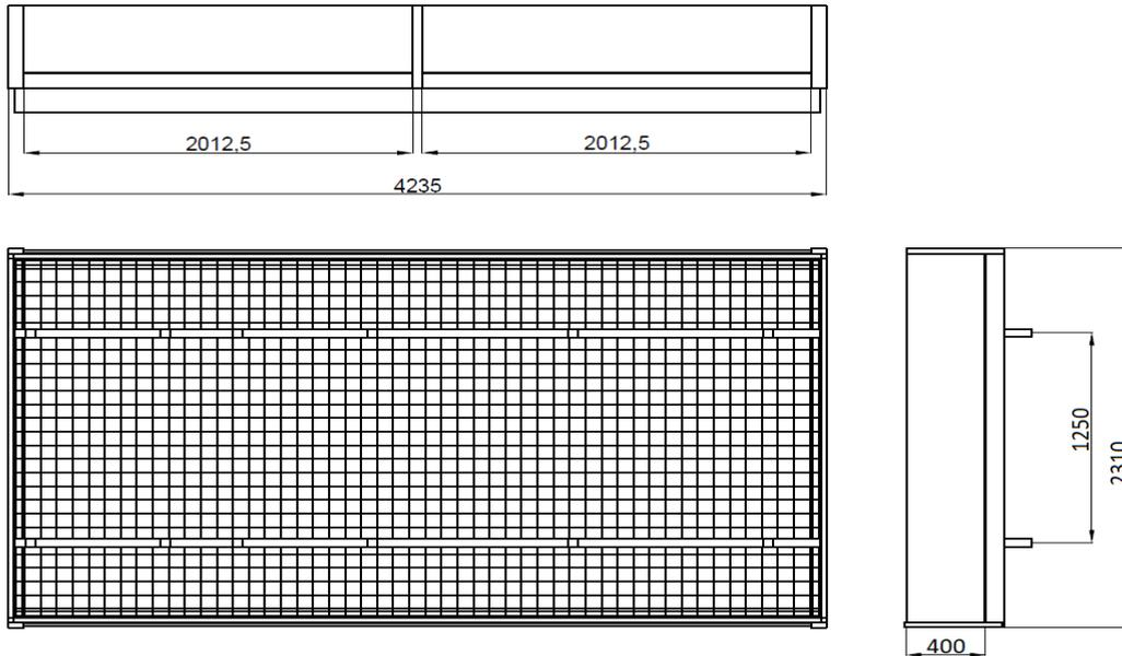
Fig. 11. Structural model of the open body designed on the basis of a grating plate
