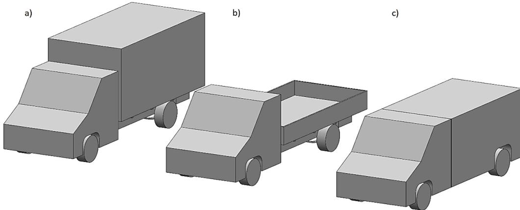
Fig. 1. Delivery vehicle body types: a - box body, b – open body, c - van body
