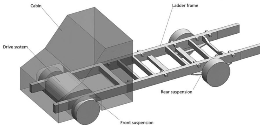
Fig. 2. Diagram of the structure of a vehicle with an independent support frame, without a transport body installed
