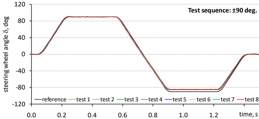
Fig. 14. Time waveforms of changes in the angular position of the steering wheel during the 90 degree turn maneuver
