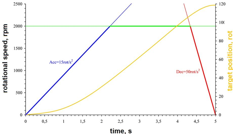
Fig. 6. Examples of servo motor motion parameters
