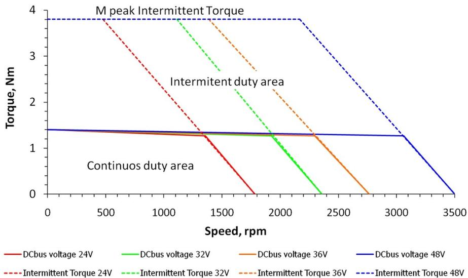
Fig. 4. Servo motor torque curve [adopted from ref. 22]
