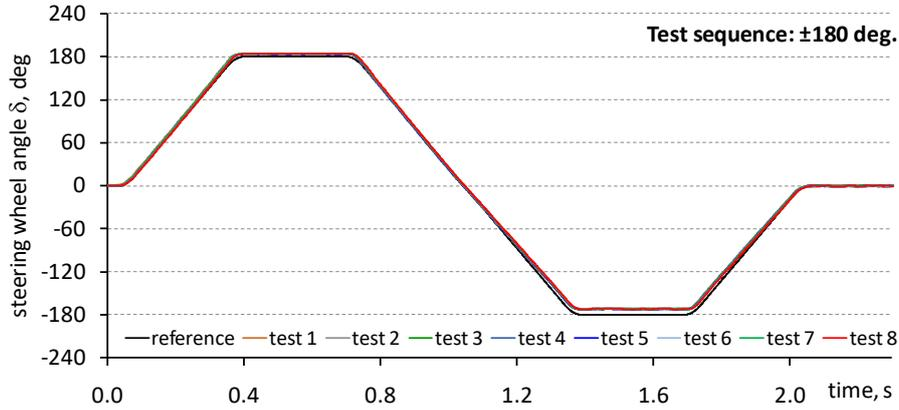
Fig. 15. Time waveforms of changes in the angular position of the steering wheel during the 180 degree turn maneuver
