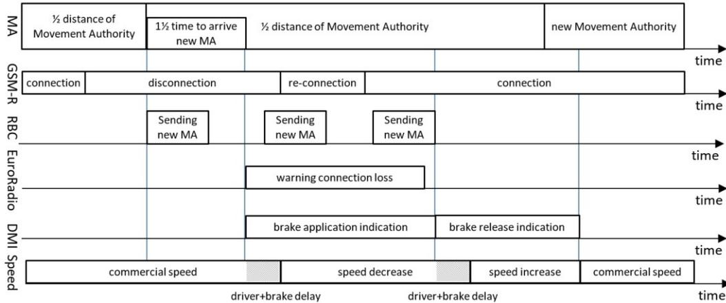
**Fig. 3. The sequence of events triggered after detection of a loss of connection with the ultimate aim of re-establishing the connection between the on-board and the RBC (based on Fig. 19 [19])**
