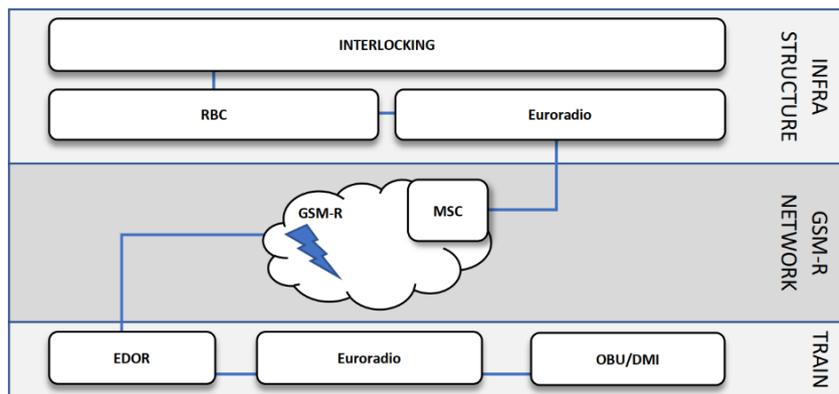
Fig. 1. Simplified ETCS communication block diagram (based on SUBSET-026, p. 2.5.3, Fig. 1 [21])
