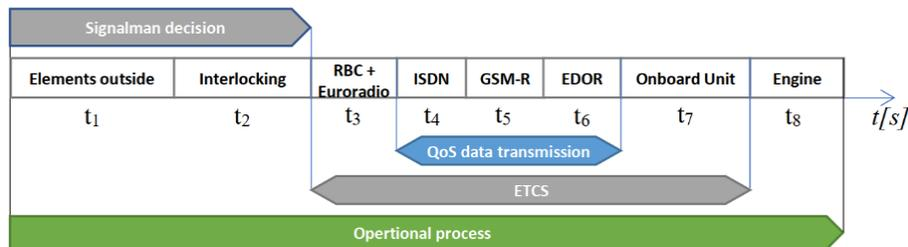
Fig. 2. Timeshare of ETCS and data-transmission of the operational process (based on [19] Fig. 1)
