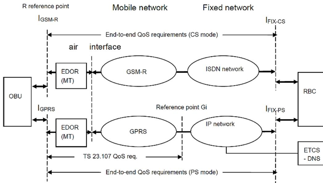
Fig. 4. The end-to-end data bearer services (based on [22] Fig. 1)
