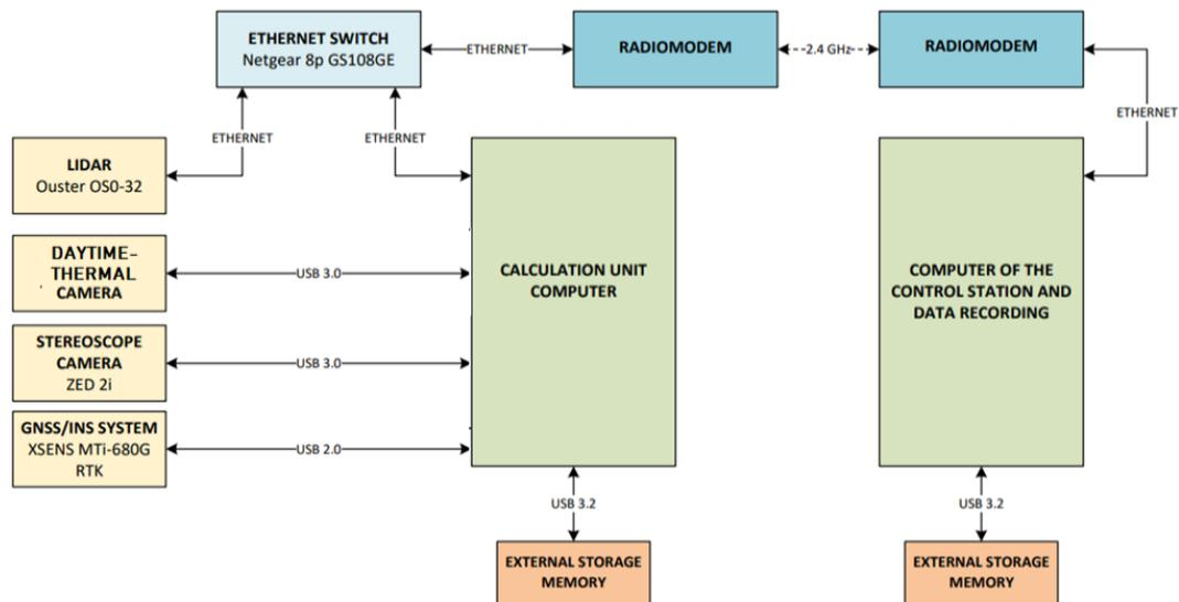
Fig. 6. Block diagram of examined perception system
