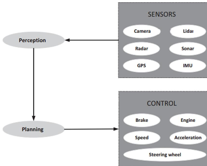
Fig. 2. Block diagram of autonomous system [19]
