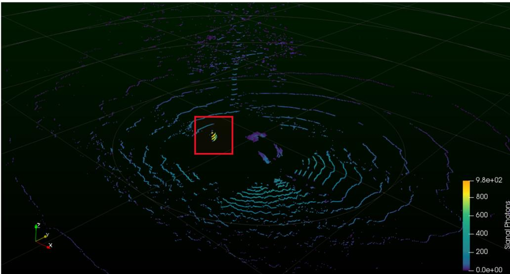
**Fig. 10. 3D environment representation of reflected energy as signal photons (The observed object is marked in red)**
