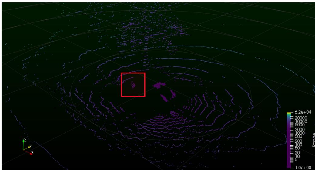
Fig. 8. 3D environment representation according to the distance from the sensor's center (The observed object is marked in red)
