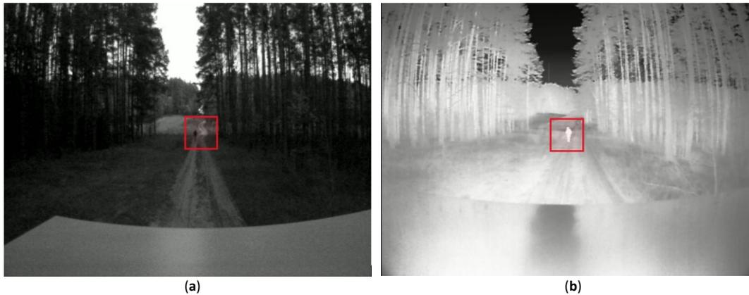
**Fig. 14. The image recorded by the RGB (a) and thermal (b) camera during night mode. The observed object is marked in red**
