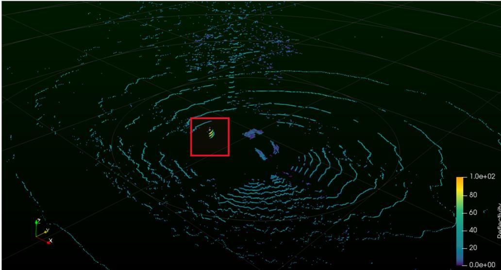
**Fig. 9. 3D environment representation measured reflection coefficient (The observed object is marked in red)**
