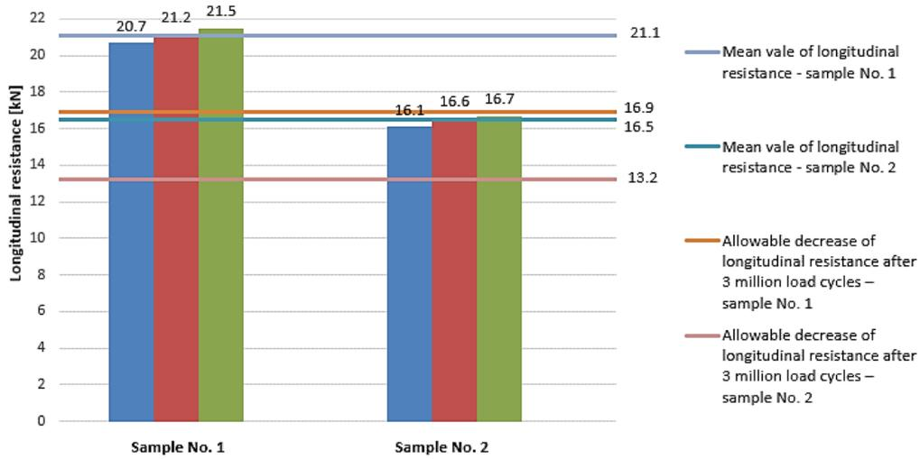
Fig. 13. Comparison of the longitudinal resistance values for the SB-type attachment for two extreme characteristics (Own source)
