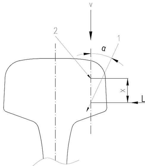
Fig. 7. Method of applying force when testing the effects of repetitive loads [2],
