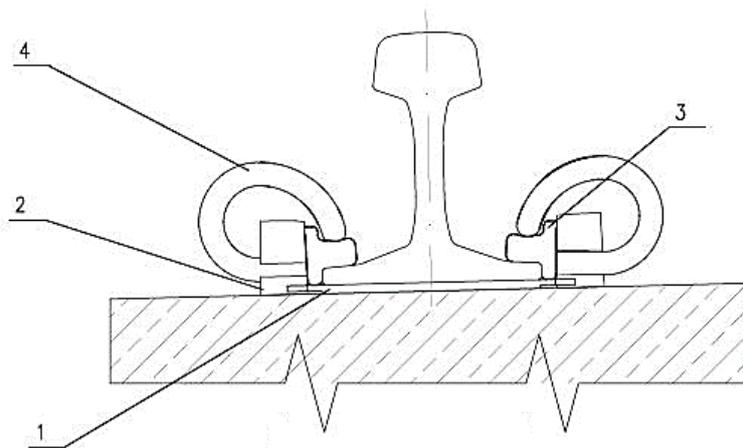
Fig. 6. Fastening system type SB. 1 – rail pad, 2 – anchor, 3 – electric insulator, 4 – SB clamp
