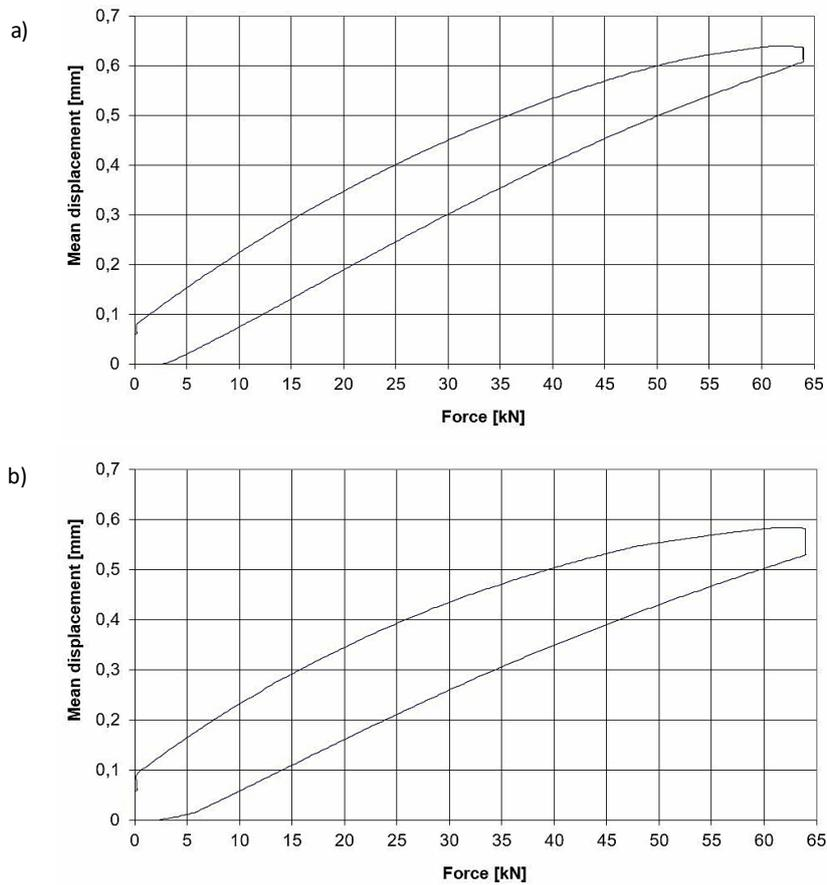
Fig. 8. Example of a force - displacement diagram for the fastening system (Own source),
