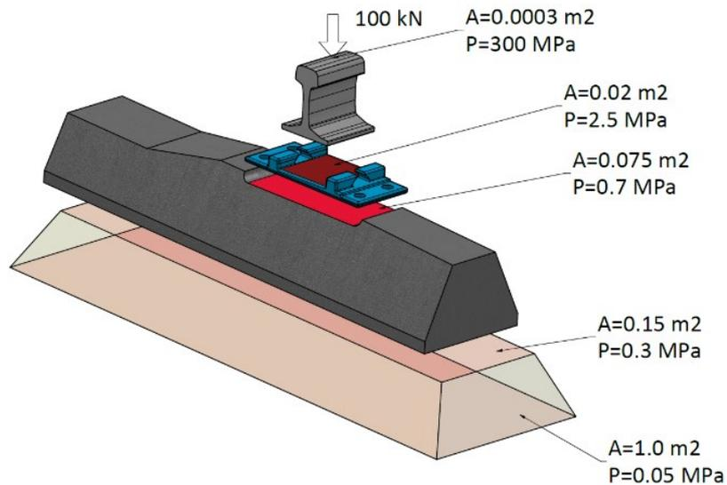
**Fig. 4. Principle of load transfer [13]**
