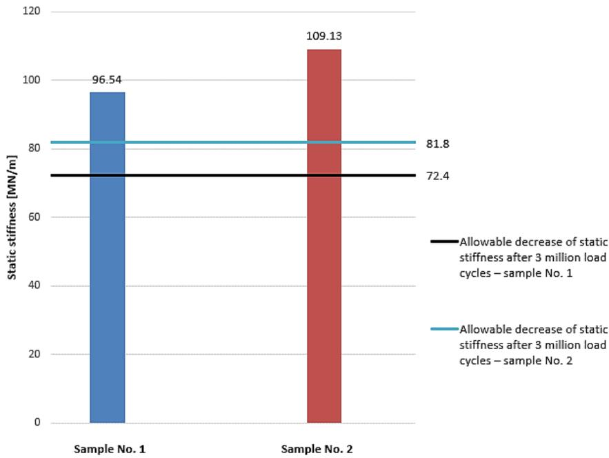
Fig. 14. Comparison of the vertical stiffness of the SB-type fastening system for the two extreme characteristics of the SB4 spring feet (Own source)
