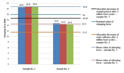
Fig. 12. Comparison of clamping force values for SB-type attachment for two extreme characteristics (Own source)
