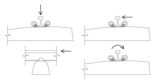
Fig. 5. Forces acting on the fastening system / railway track [5]
