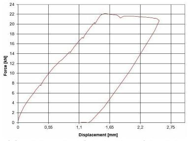
Fig. 11. Example of a force - displacement diagram for sample 1 in the case of a longitudinal resistance test [10]
