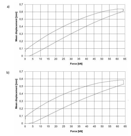
Fig. 8. Example of a force - displacement diagram for the fastening system (Own source), Sample 1 – clamp stiffness SB C = 1,52 kN/mm, Sample 1 – clamp stiffness SB C = 1,18 kN/mm
