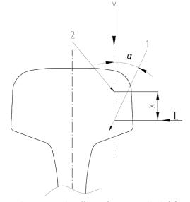
Fig. 7. Method of applying force when testing the effects of repetitive loads [2], 1 - line of load application, 2 - centre of gauge corner radius
