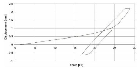
Fig. 10. Example force - displacement diagram for sample 1 in the case of clamping force test (Own source)
