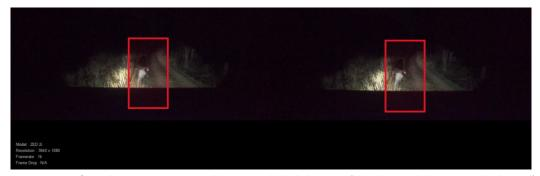
Fig. 13. Image from the ZED2i camera - night view - vehicle lighting on (The observed object is marked in red)
