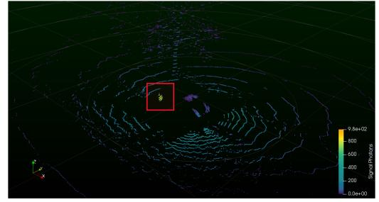
Fig. 10. 3D environment representation of reflected energy as signal photons (The observed object is marked in red)
