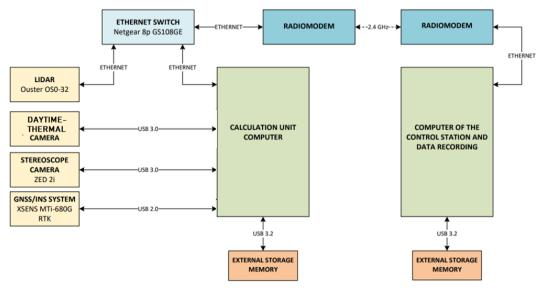
Fig. 6. Block diagram of examined perception system
