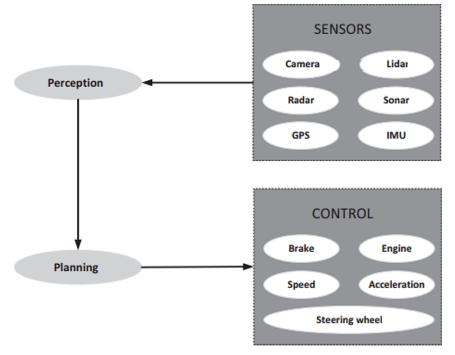
Fig. 2. Block diagram of autonomous system [19]
